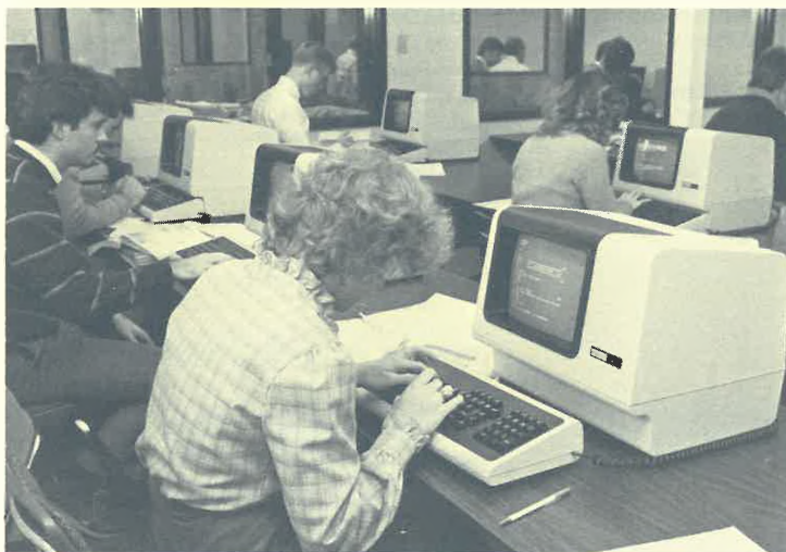
Cedarville College academic computer facilities include a DEC VAX 11/750 minicomputer. Adjacent to the computer room are 17 terminals in a student and faculty lab which provide direct access to the VAX.
