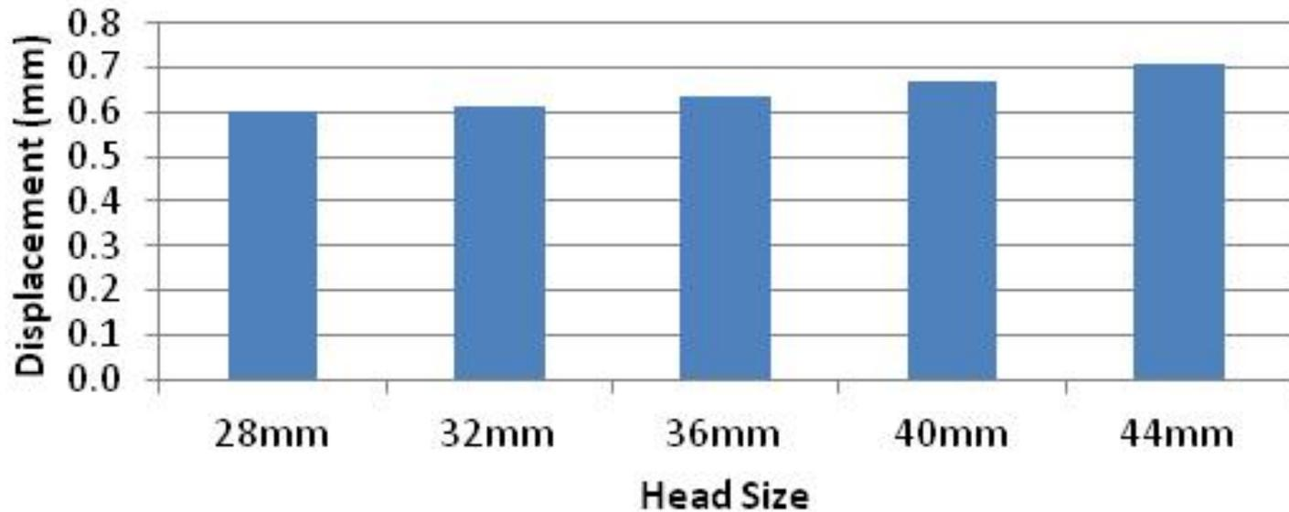
**Figure 3:** *Motion of the femoral head relative to the neck of the 12/14 tapered implant.*
