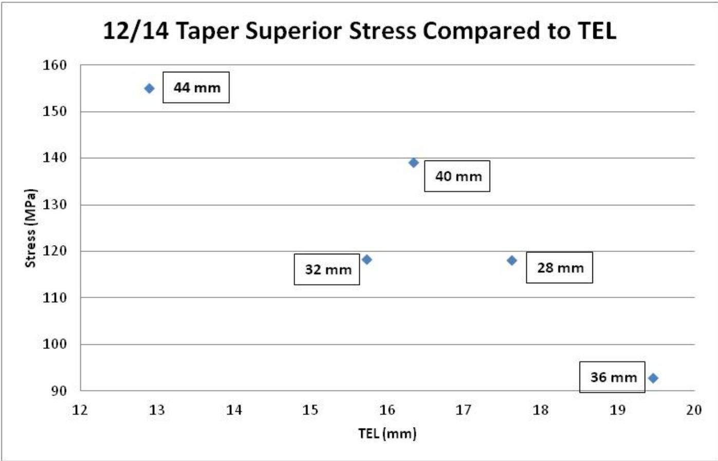
**Figure 6:** *Stresses on the superior face of the 12/14 tapered implant in comparison to the TEL of the head. Head sizes shown in box next to the data point.*
