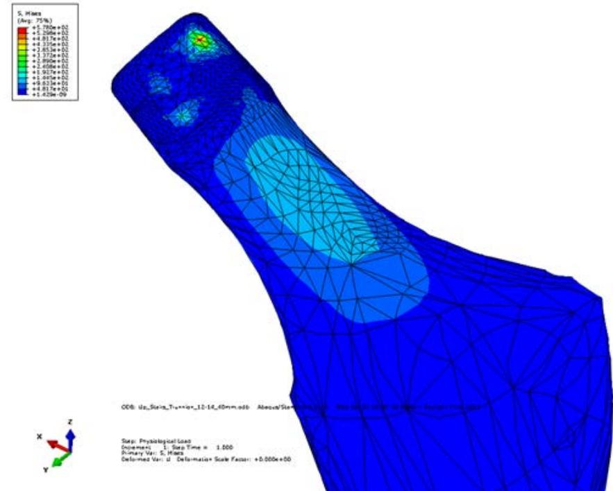
**Figure 1:** *Finite Element Model Results. The red area indicates the location of highest stress while the blue indicates a point of lower stress*
