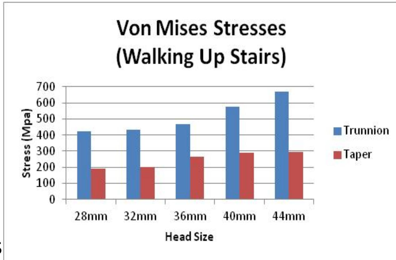
**Figure 2:** *Maximum Von Mises stresses on the taper and trunnion of a 12/14 taper implant.*
