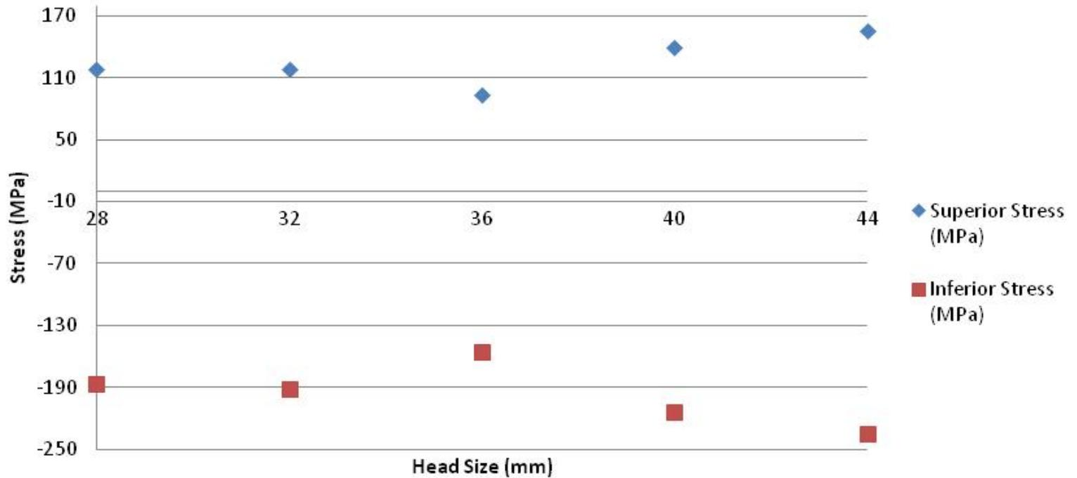
**Figure 5:** *Stresses on the superior and inferior faces of the implant compared to the size of the femoral head*
