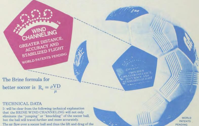
The air flow over a soccer ball and thus the lift and drag of the ball are dependent on whether the local boundary layer is laminar or turbulent, i.e. whether the flow is so-called subcritical, transcritical or supercritical.
