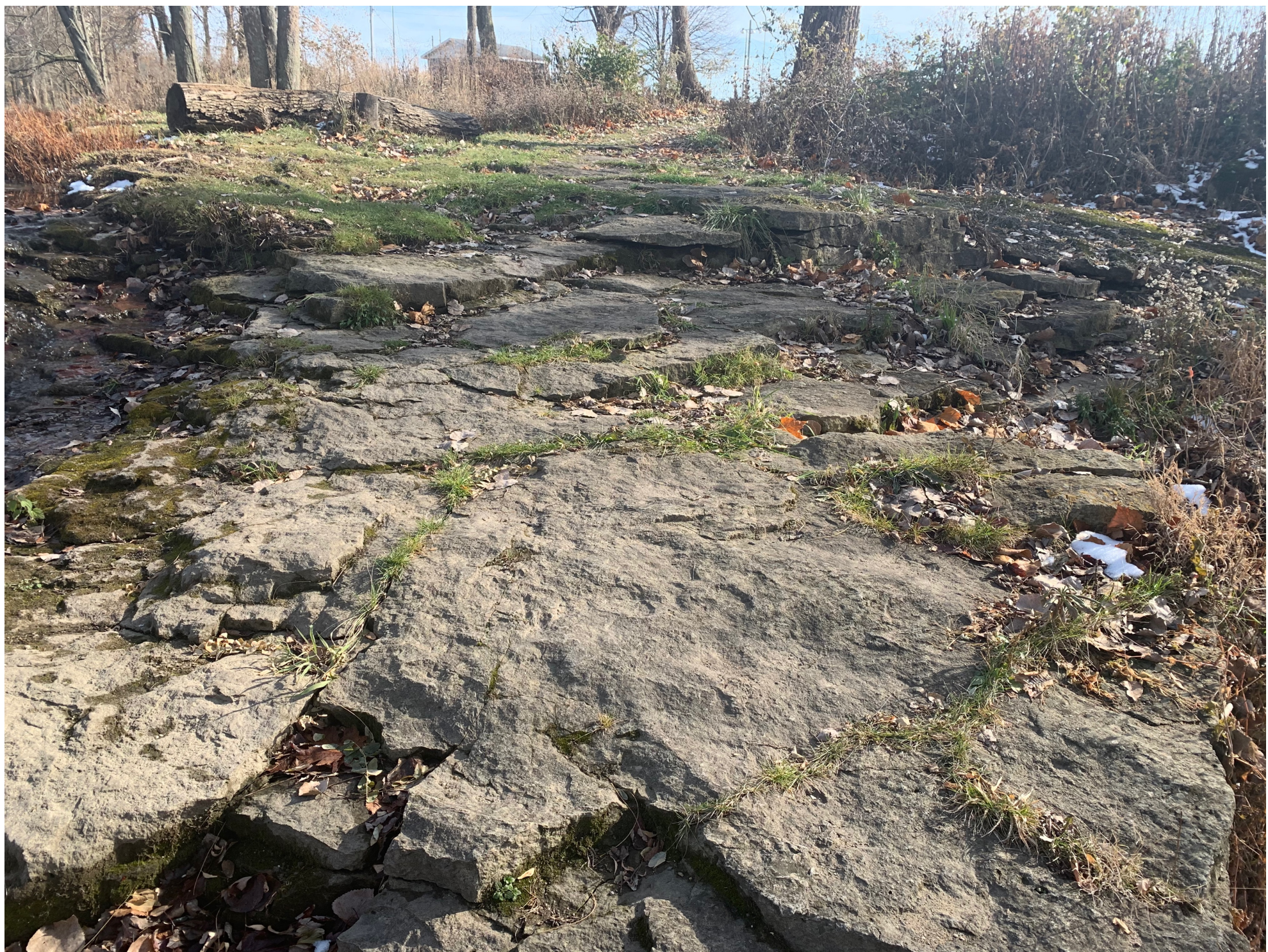
Fig.3: Exposed bedrock from site 2. Note the lines of grass marking the locations of joints.
