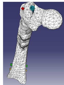
Figure 1. Finite element model of implanted intramedullary nail
