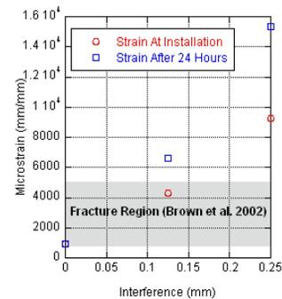
Figure 2. Cortical bone circumferential strain due to press-fit of nail
