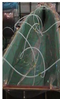
The hull being manufactured using a vacuum infusion process to draw resin through the Kevlar fibers
