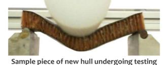
Sample piece of new hull undergoing testing
