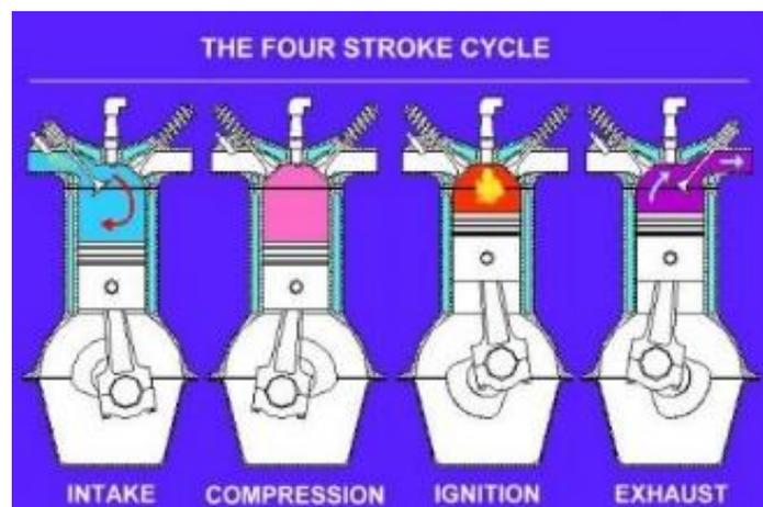
After that is the compression stroke, during which the valve is closed and the piston moves up,
