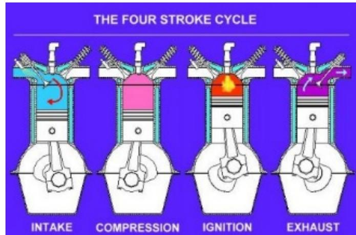
The first cycle is the intake stroke, in which the piston is moving into the cylinder top. At the same time, fuel is injected into the chamber, forming a mixture of air and fuel.
