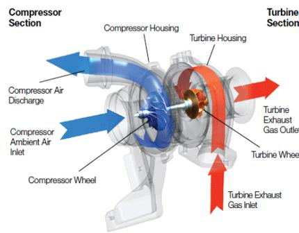
proportionately higher amount of fuel. The obvious benefit here is the direct increase in the engine power; at the same time, down-sizing of the engine is possible” (Giakoumis 2016). Below is a graphic showing air routing through an engine and turbocharger system, as well as specific air routing through the turbocharger itself.
