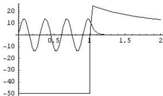
Figure 5: The Exponentially Diffuse boundary potential and the corresponding wavefunction. The vertical axis is energy in MeV and the horizontal axis is the radius  $\rho$ . For the wavefunction, the vertical axis is the real part of the wavefunction multiplied by ten.
