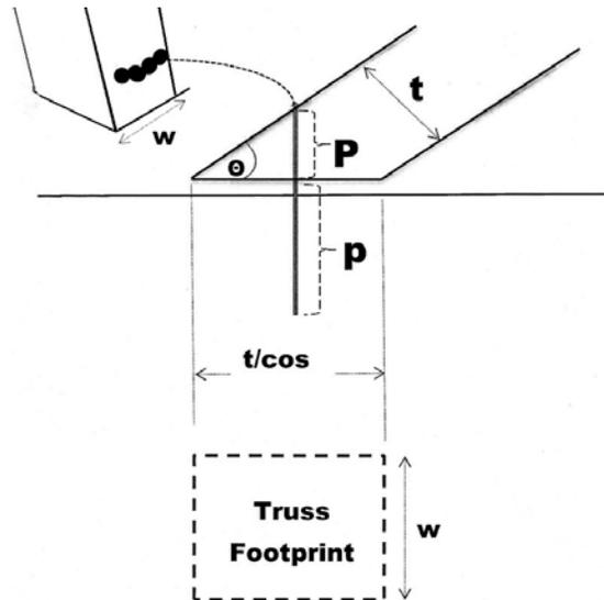
**Figure 3.** View in profile of web/floor/joint detail: Web-member thickness ( $t$ ), width ( $w$ ), and angle to Ark-floor chord ( $\theta$ ); dowel-penetration depth in web member ( $P$ ) and floor ( $p$ ).
