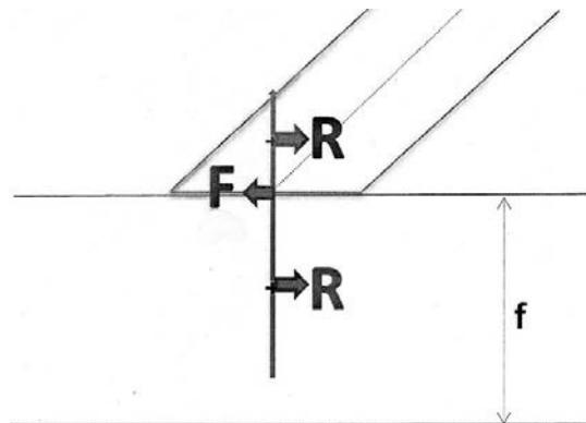
**Figure 4.** Eccentric web-chord joint: Force ( $F$ ), reaction ( $R$ ), and floor thickness ( $f$ ).
