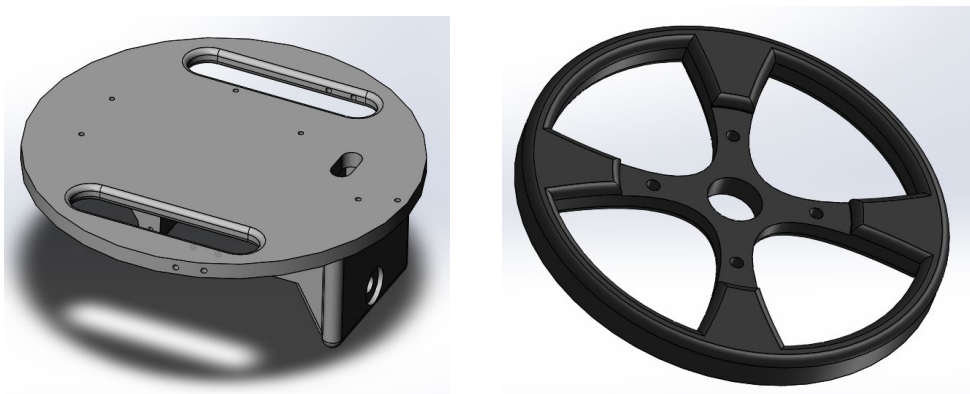
Figure 2. SolidWorks renderings of the chassis and wheels given to the students.
