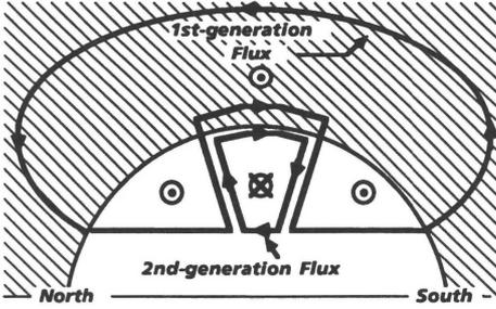
Figure 8(b). New flux is generated.
