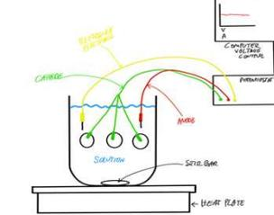
Figure 1. Electrodeposition Experiment Set-Up
